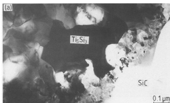
Figure 8 Reacted for a longer time 900°C, 100 h. (a) Bright-field micrograph; (b) diffraction pattern.
